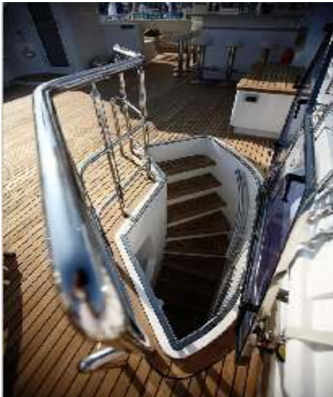
Aluminum Staircase into F/B w/hatch cover
