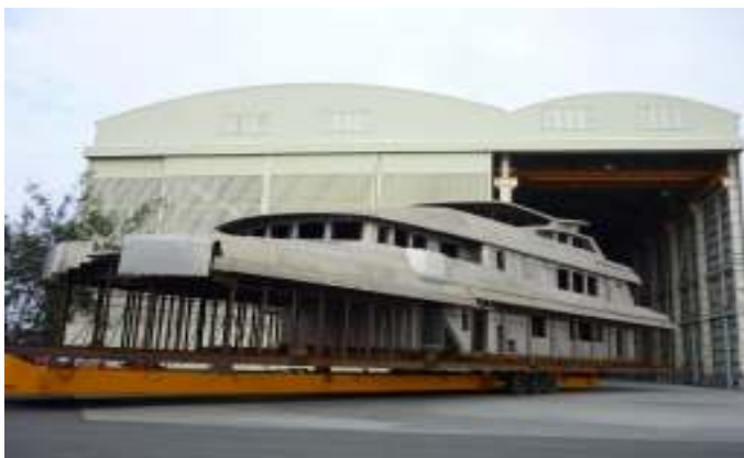
Aluminum Alloy Superstructure
